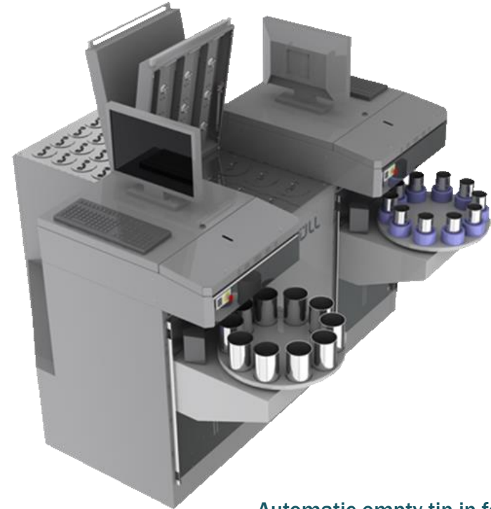
Automatic empty tin in-feed system with carousel
